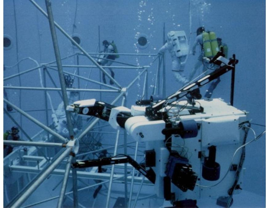
Robotic Assembly of EASE and other structures in neutral buoyancy.
